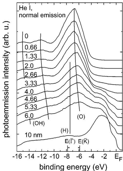
FIG. 3. Photoemission spectra of Pd covered polycrystalline yttrium films taken in UHV after exposure to 1800 L H<sub>2</sub>. (OH) and (O) are attributed to yttrium hydroxide and oxide states, respectively.  $E(\bar{\Gamma})$ ,  $E(\bar{K})$  indicate the energies of the hydrogen induced split-off states on Pd(111).<sup>33</sup>
