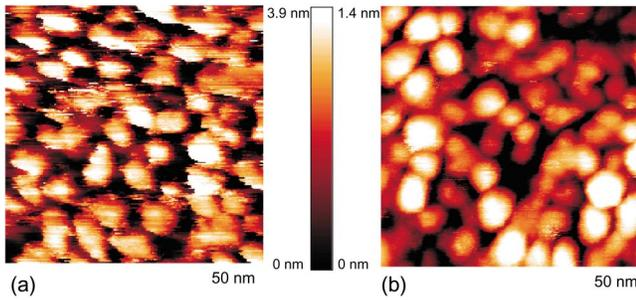
FIG. 5. Topography images of Pd clusters on Y(0001) on  $\text{CaF}_2$  (111), directly after growth (a) and after exposure to  $10^{-4}$  mbar hydrogen for 1 h (b), acquired at  $U_{\text{gap}}=5$  V,  $I=0.5$  nA and  $U_{\text{gap}}=1$  V,  $I=0.5$  nA, respectively. The nominal Pd thickness is 3 nm.
