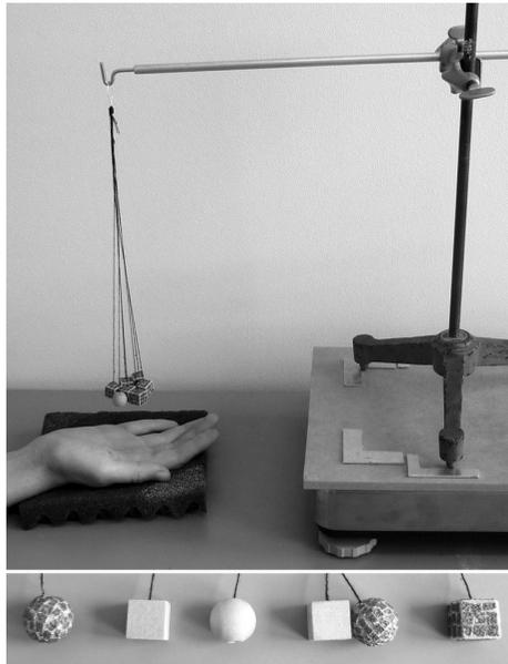
**Figure 5.1:** The experimental set-up. A bundle hangs from the tripod that is placed on the weighing scale. The close-up below shows the targets for the four conditions: sphere, smooth, combi and 2-targets, and the distractor in all conditions.
